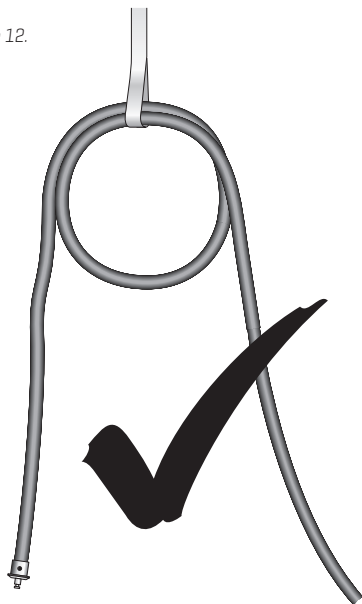
Correct method of hoisting HVSC Plus
